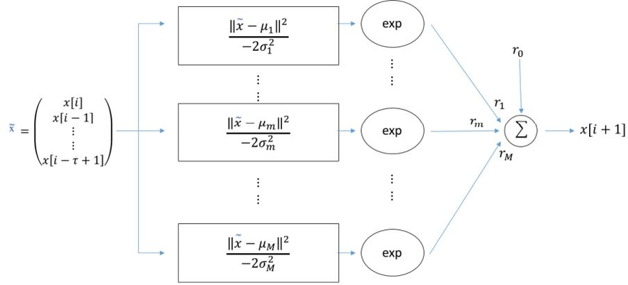
FIGURE 5. An RBF multilayer neural network model with  $L=1$
