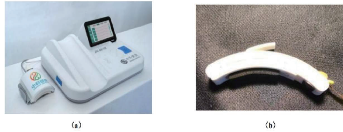
FIGURE 2. (a) Multi channel pulse wave acquisition device. (b) A compound pressure sensor.
