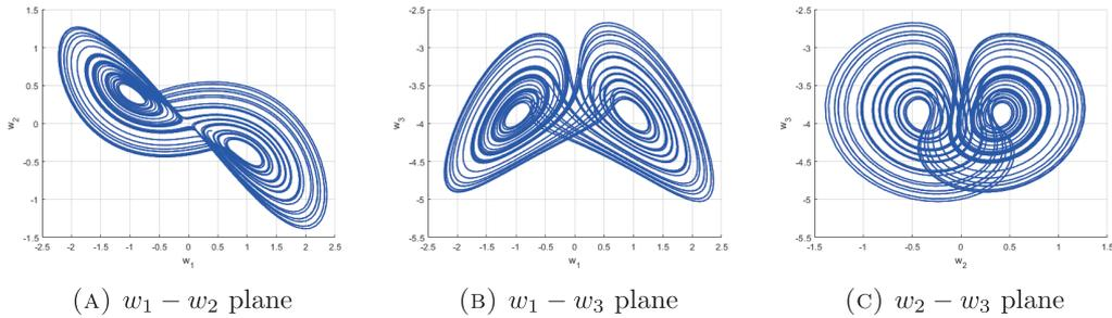
FIGURE 2. (A), (B) and (C) denote the phase portraits of the 3D chaotic system (2.2) with  $\mu = 2.5$ ,  $\beta = 0.3$ ,  $\kappa = 4$  and  $\delta = 0.1$
