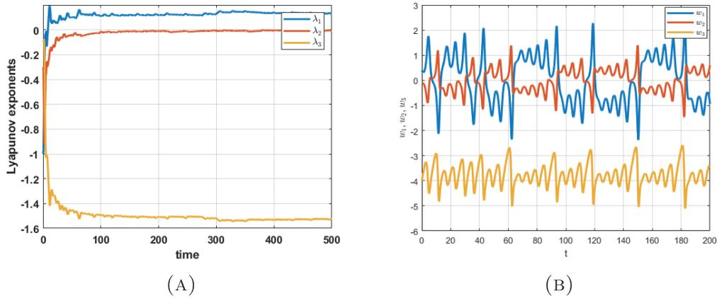
FIGURE 1. (A) Lyapunov exponents; (B) Time Series of the system (2.2) with  $\mu = 2.5$ ,  $\beta = 0.3$ ,  $\kappa = 4$  and  $\delta = 0.1$
