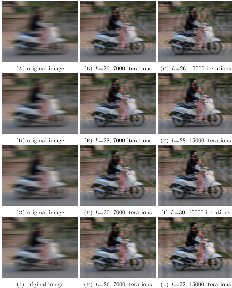
FIGURE 1. Images restored using different motion blur lengths L and iteration.
